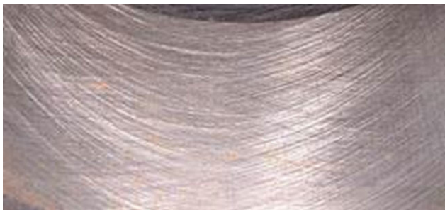
Fig.2: New honing profile and crosshatching with the right angle
